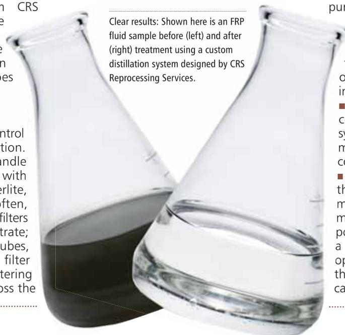
Clear results: Shown here is an FRP fluid sample before (left) and after (right) treatment using a custom distillation system designed by CRS Reprocessing Services.
